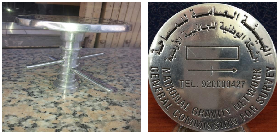
Figure 5: Survey Marker for Absolute Gravity Station (Source: GEOSA Geodetic Guidelines ( General Authority for Survey and Geospatial Information, GEOSA, 2024 )).
