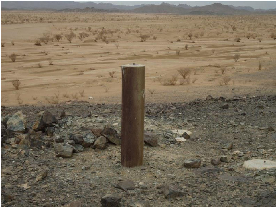
Figure 10: Geodetic pillar type 2
