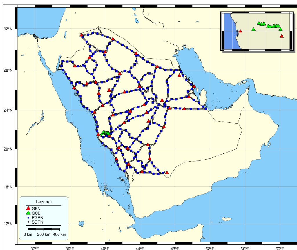
Figure 3: National Gravity Network (Source: SANSRS Technical Summary ( General Authority for Survey and Geospatial Information, GEOSA, 2022 )).
