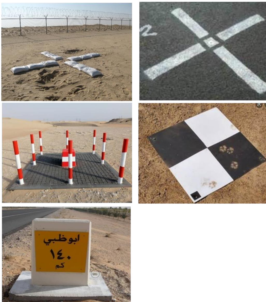
Figure 10: Examples of Premark Ground Control Points
